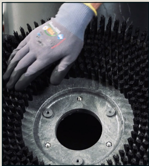
Press the brush click off button and inspect the brush or pad
