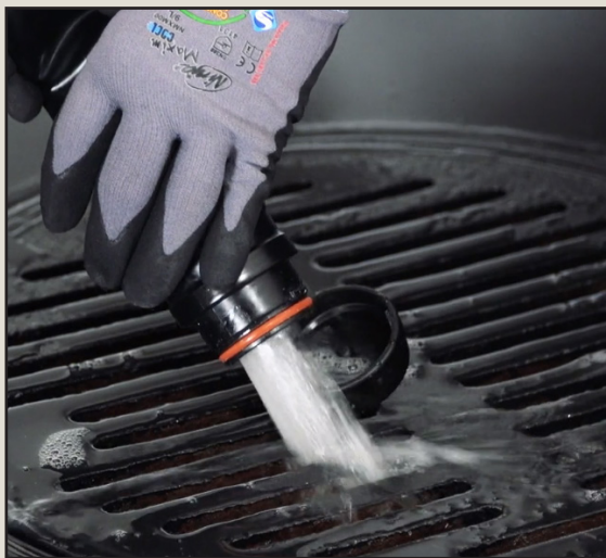
Empty and clean the recovery tank and floating system
