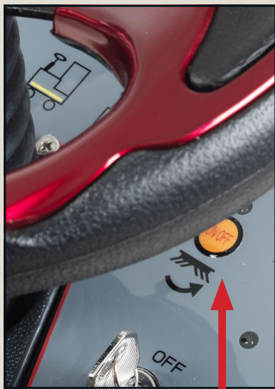
Press the brush click off button and inspect the brush or pad
