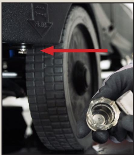
Empty solution tank. Check and clean filter (weekly)
