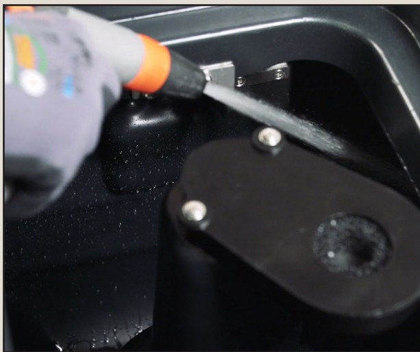
Empty and clean the recovery tank and floating system
