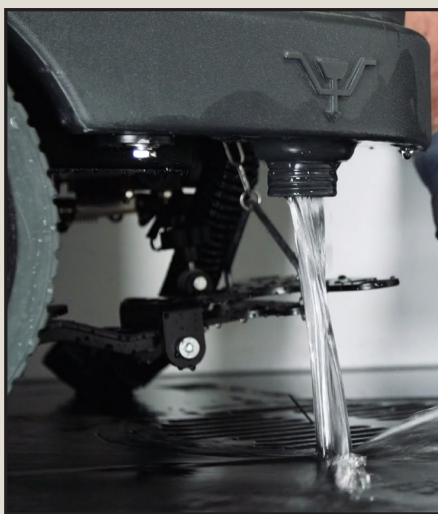
Empty solution tank. Check and clean filter (weekly)
