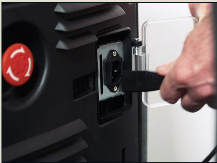
Connect battery charger to socket
